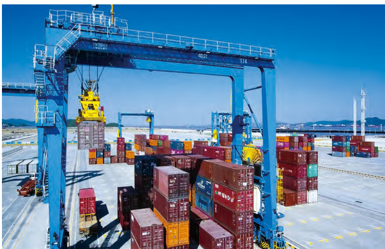
■ China's first 5G+ remote control gantry crane was put into use in Ningbo Zhoushan Port
